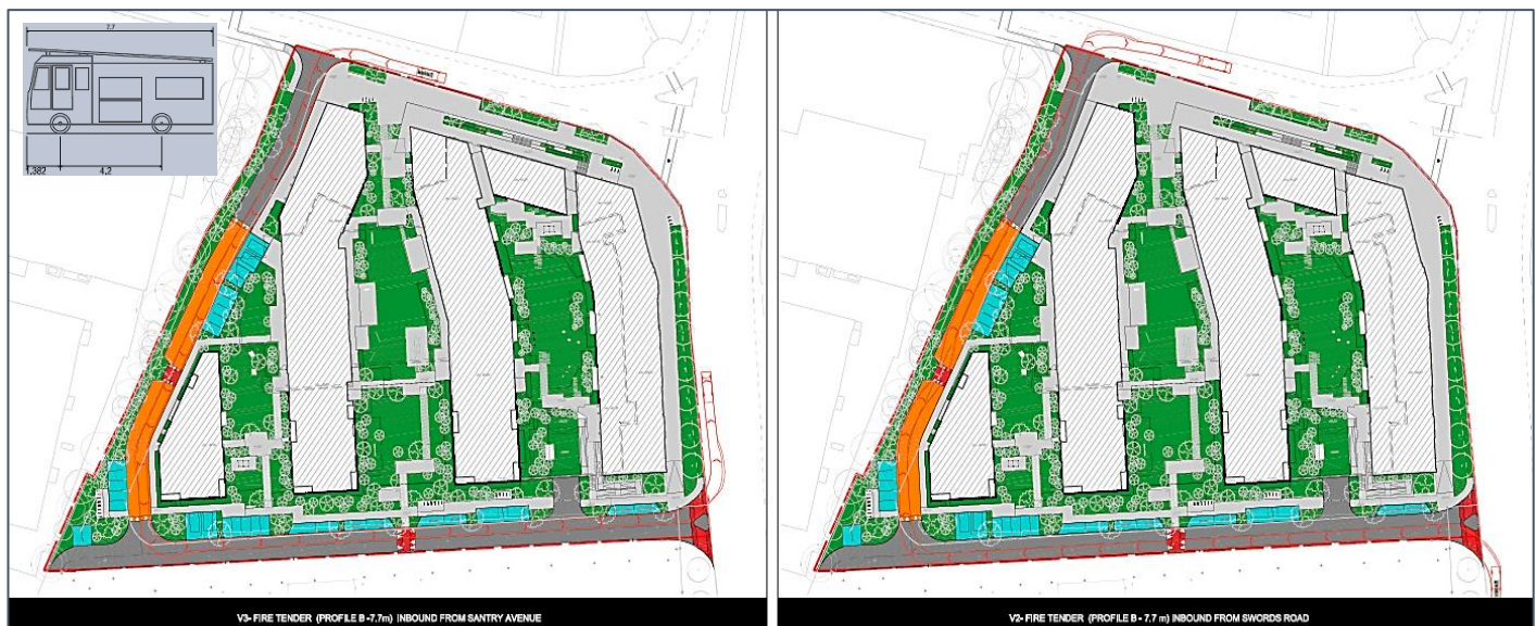
Figure 4-5: Swept Path Analysis for a Fire Tender
