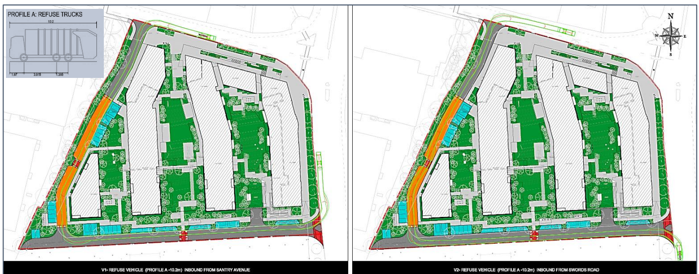
Figure 4-3: Swept Path Analysis for Refuse Vehicle
